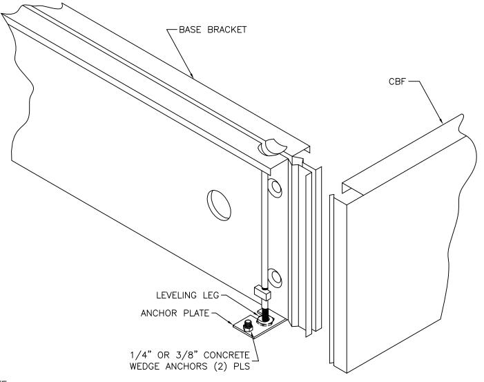
NOTE: FOR POSITIONING APPLICATIONS, USE WEDGE ANCHORS WITH 1 1/8 MINIMUM EMBEDMENT. FOR SEISMIC APPLICATIONS, CONSULT A SEISMIC ENGINEER FOR SPECIFIC ANCHOR SIZE/TYPE INSTALLATION DETAILS.
