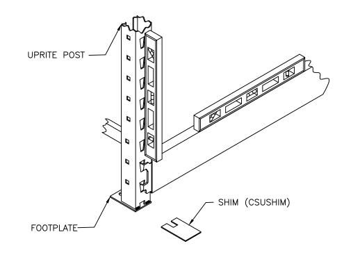
STEP 2. Use shims to level the system as required for uneven floors.
