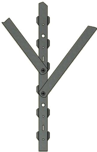
Where adjacent sections have braces, offset the braces (1) hole on the common upright
